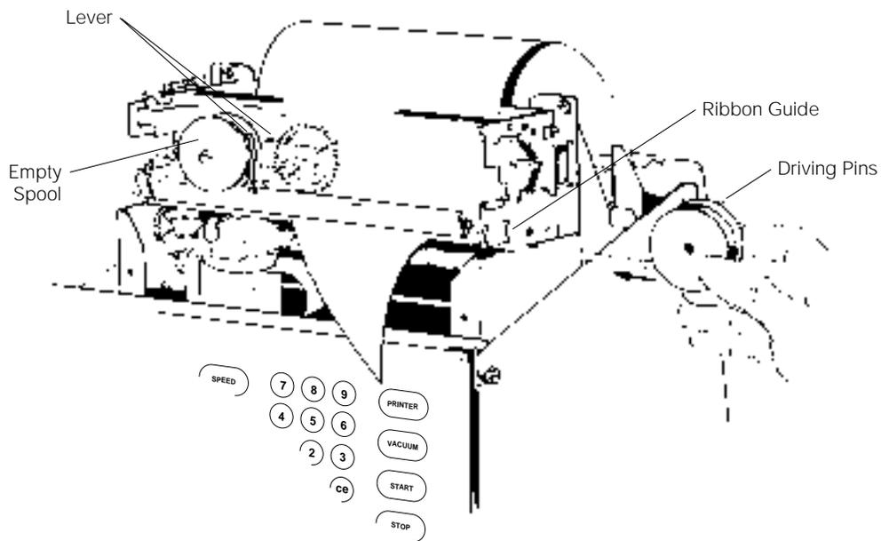
Figure 9-9. Inserting the New Ribbon
