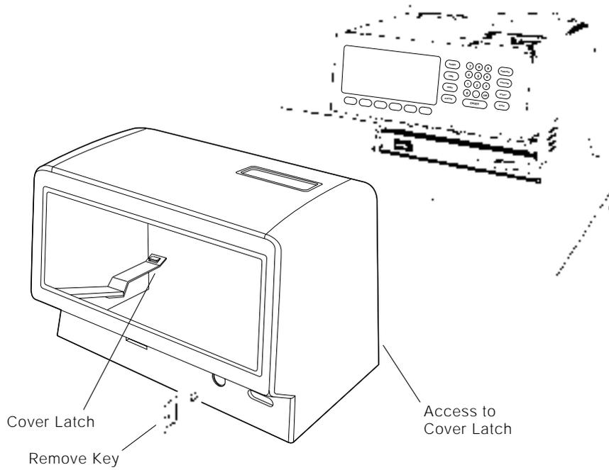
Figure 9-1. Removing the Control Head Cover
