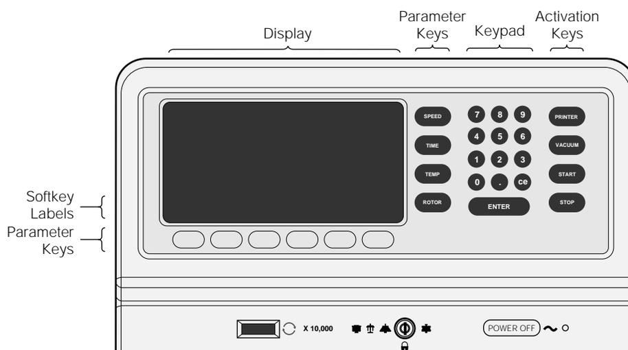
Figure 1-3. The Control Panel
