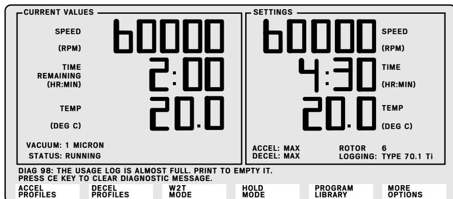
Figure 9-5. Screen with a Diagnostic Message Displayed
