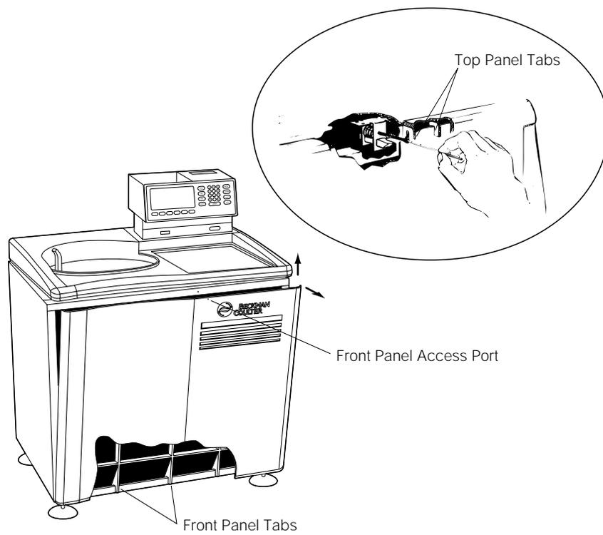
Figure 9-2. Depressing the Latch to Loosen the Front Panel
