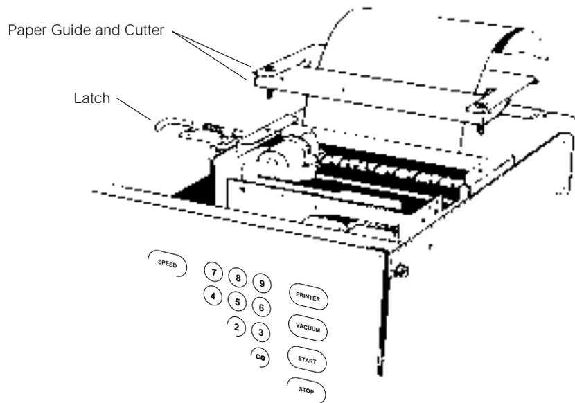
Figure 9-8. Removing the Paper Guide and Plastic Cutter
