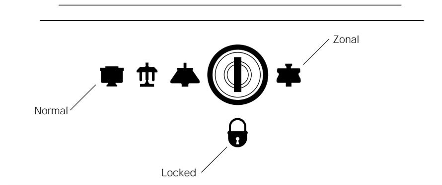
Figure 1-2. Key Switch Positions
