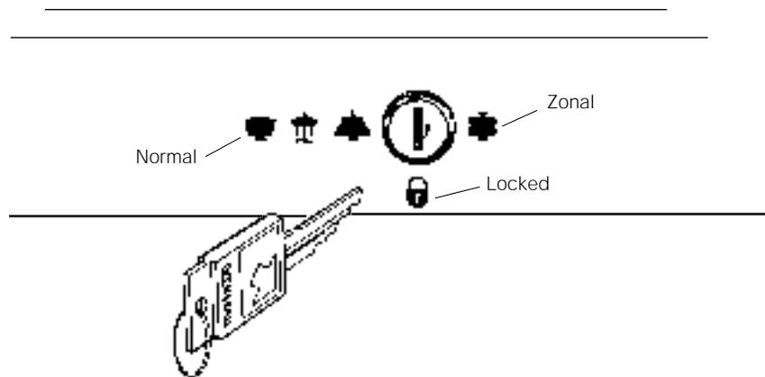
Figure 2-5. Inserting the Key into the Interlock Switch
