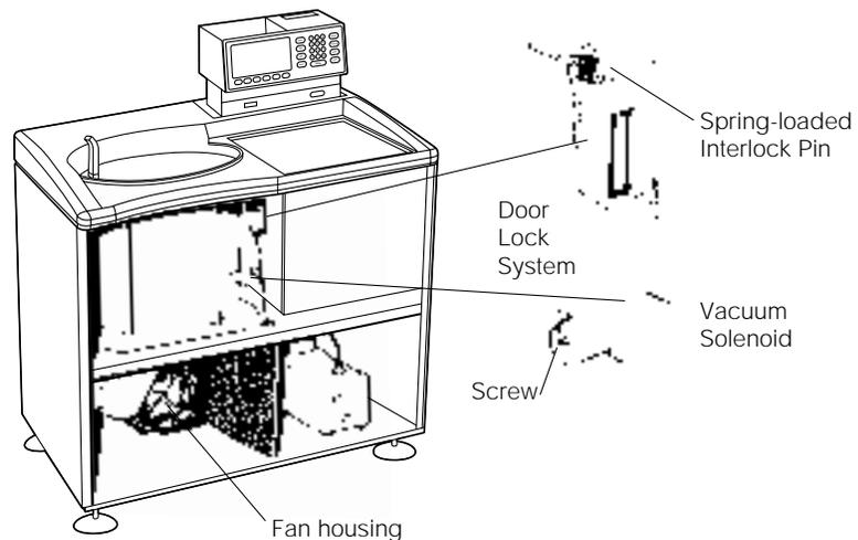
Figure 9-3. Interior View of Instrument (Panel Removed)
