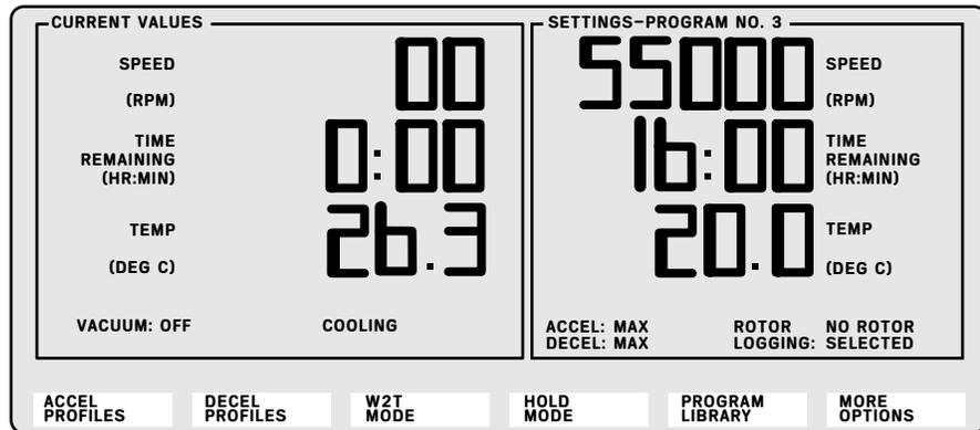
Figure 3-2. Entering an Existing Program for Use
