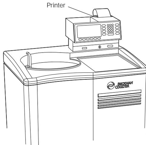
Figure 1-4. Location of Printer Within Control Head
