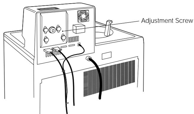
Figure 9-6. Location of the Screw that Adjusts Video Brightness
