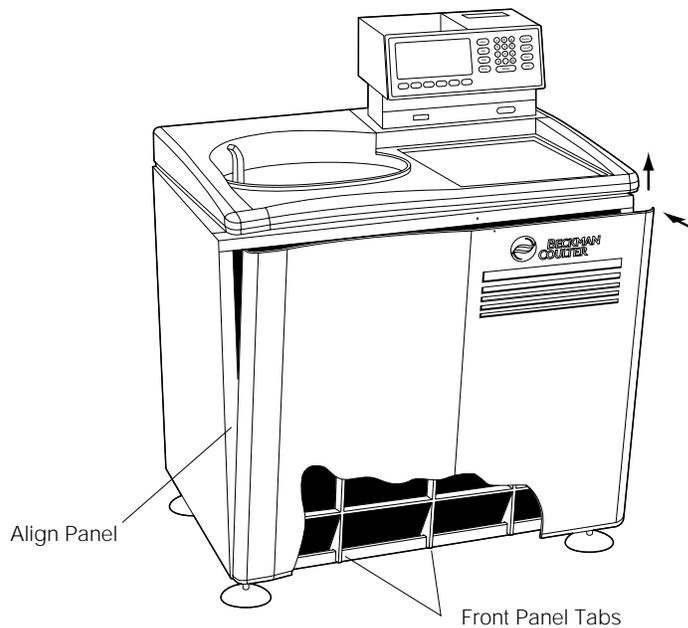
Figure 9-4. Reinstalling the Front Panel
